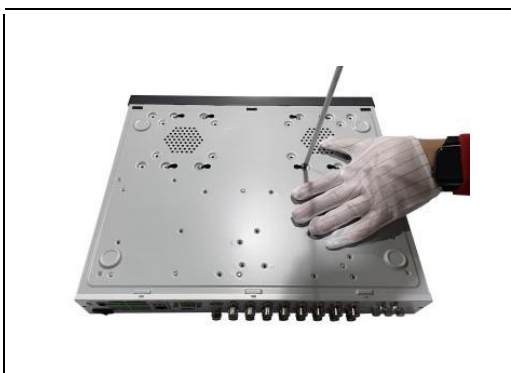
Figure 1-3-2 Fix the HDD
