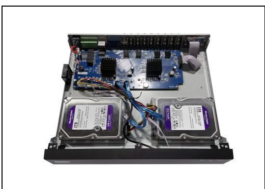
Figure 1-3-3 Connect the power and data cables
