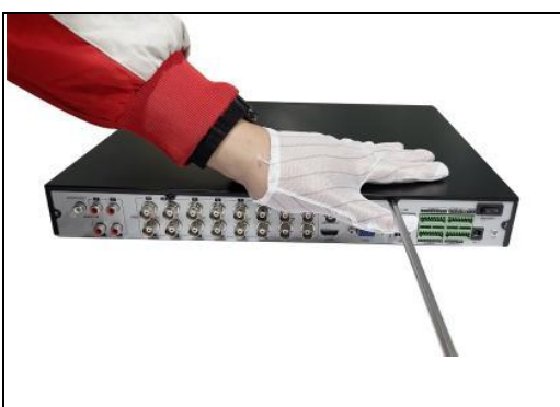
Figure 1-3-4 Install the cover and screws
