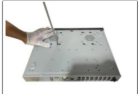
Figure 1-19 Fix the HDD
