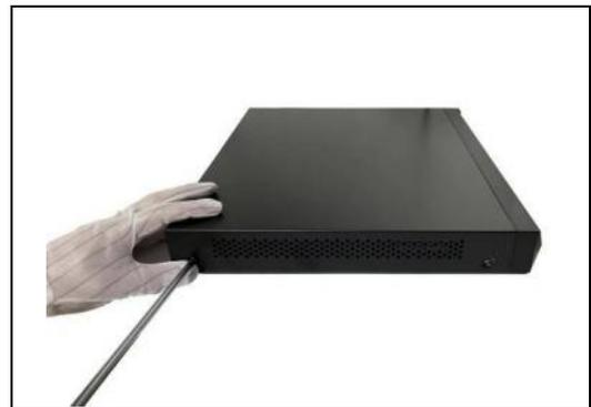
Figure 1-21 Install the cover and screws
