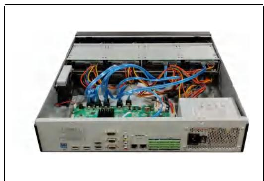
Figure 1-23 Connect the power and data cables
