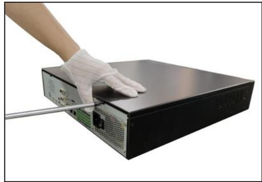
Figure 1-25 Install the cover and screws
