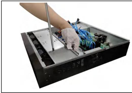
Figure 1-24 Fix the HDD
