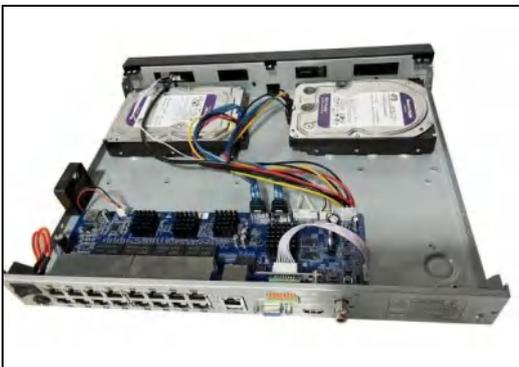
Figure 1-20 Connect the power and data cables
