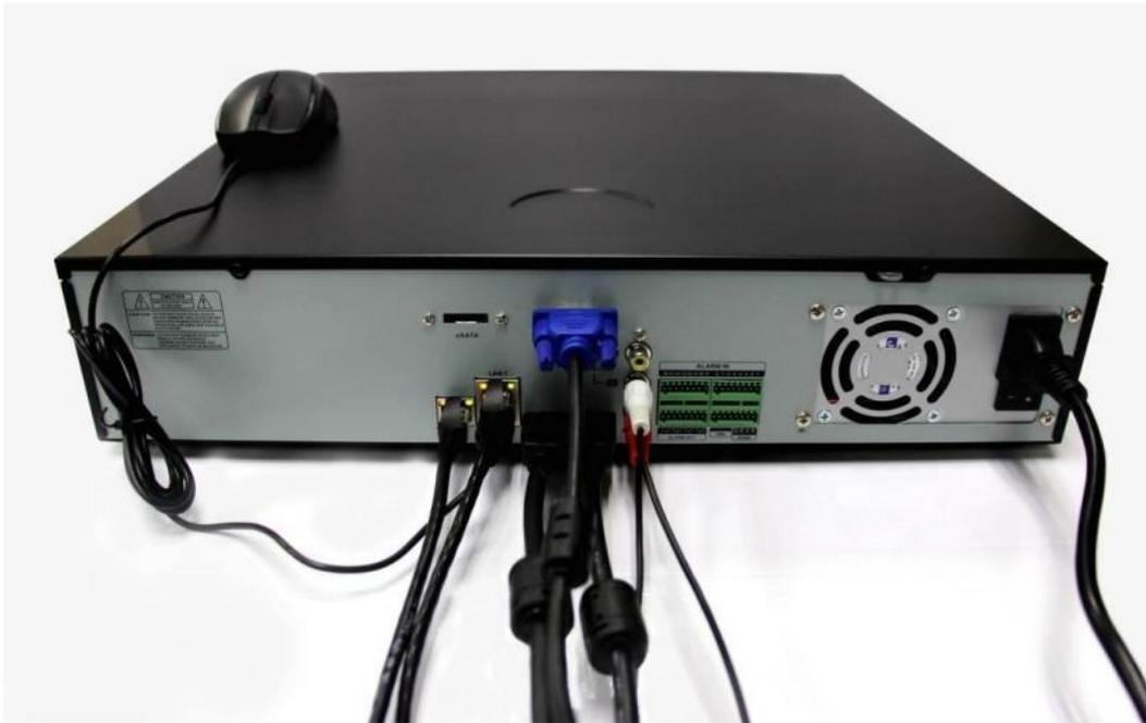
Figure 1-31 Power Supply Connection
